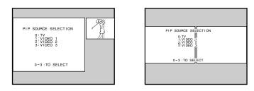
While the above menu is on the screen, you can select the desired signal input source by pressing the corresponding number button (0-3).
